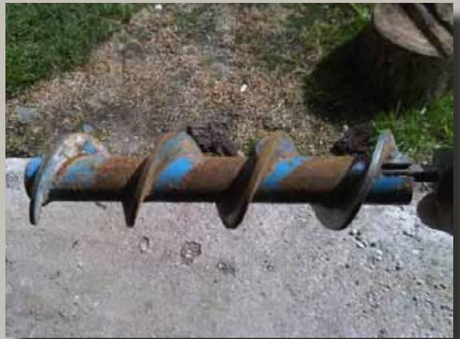
Rotating hammers after they get rounded. Feeling screens and replacing when worn. Replacing worn out equipment and checking supply augers for build up especially after humid weather.
